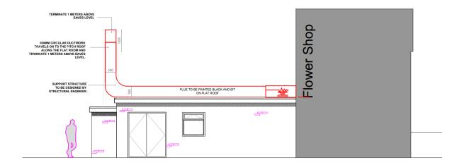
The flue/extract has now been designed to ensure the output pipe is above the existing eaves height of the neighbouring properties and the system now incorporates advanced filtration systems within it to ensure the neighbouring residents and units are not detrimentally affected by any smells or noise. The applicants submitted noise assessment concludes that:
